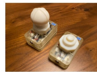
Hardware design incorporating a six-axis tactile sensor to allow users to operate ICT terminals using few force.
