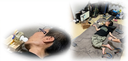
Hardware design incorporating a six-axis tactile sensor to allow users to operate ICT terminals using few force.
