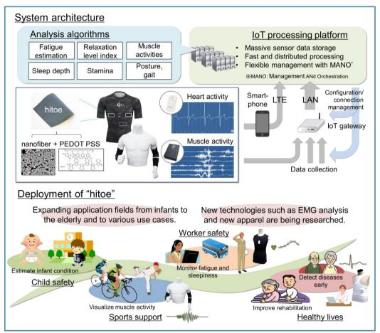
"hitoe", a functional textile created by NTT and Toray, is integrated with clothes and enables the measurements of heart and muscle activities by just wearing them.
