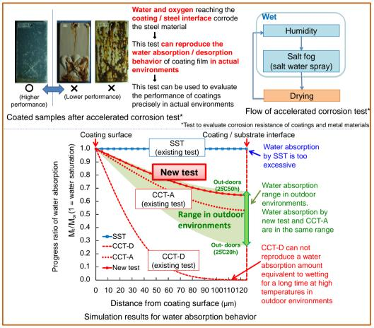
A new accelerated corrosion test for evaluating the corrosion resistance of coatings was designed to approximate the water absorption and desorption behavior of coatings in outdoor environments. The test can well approximate atmospheric corrosion in seafront areas and accelerate corrosion by 1.4 times or more compared with existing tests. This test enables us to accurately select long-life coatings in a shorter test time.
