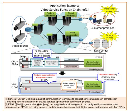
The current CPU+FPGA architecture has a large communication overhead between the CPU and FPGA. This issue currently prevents FPGAs from being used in some cloud services. Our FPGA accelerator solves the problem and enables low-latency and high-throughput cloud video services by streaming pixel-related calculations encapsulated in packets.
