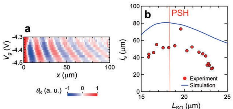
Fig. 2. (a) Gate voltage dependence of the spatial distribution of drifting spins in the [1-10] direction. (b) Spin decay length  $l_s$  as a function of spin rotation length  $L_{SO}$  in which an electron spin can rotate a full cycle.
