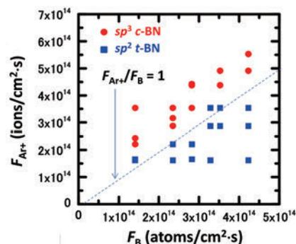
Fig. 3. Growth phase diagram for BN as functions of  $F_{Ar^+}$  and  $F_B$ .
