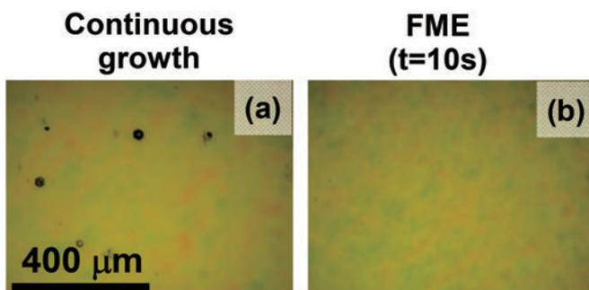
Fig. 1. Optical micrographs of the surfaces of N-face GaN (000 $\bar{1}$ ) films grown by (a) conventional continuous growth ( $t = 0$ ) and (b) group-III-source FME ( $t = 10$  s).
