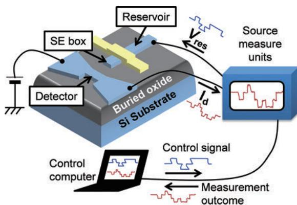
Fig. 1. Schematics of feedback control of SEs. Number  $n$  of SEs in the SE box is monitored with current  $I_d$  through the detector (red line). Voltage  $V_{res}$  applied to the electron reservoir was modulated based on the  $n$  measurement outcome (blue line).
