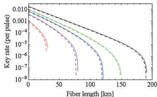
Fig. 1. Communication distance vs Key generation rate per pulse.
