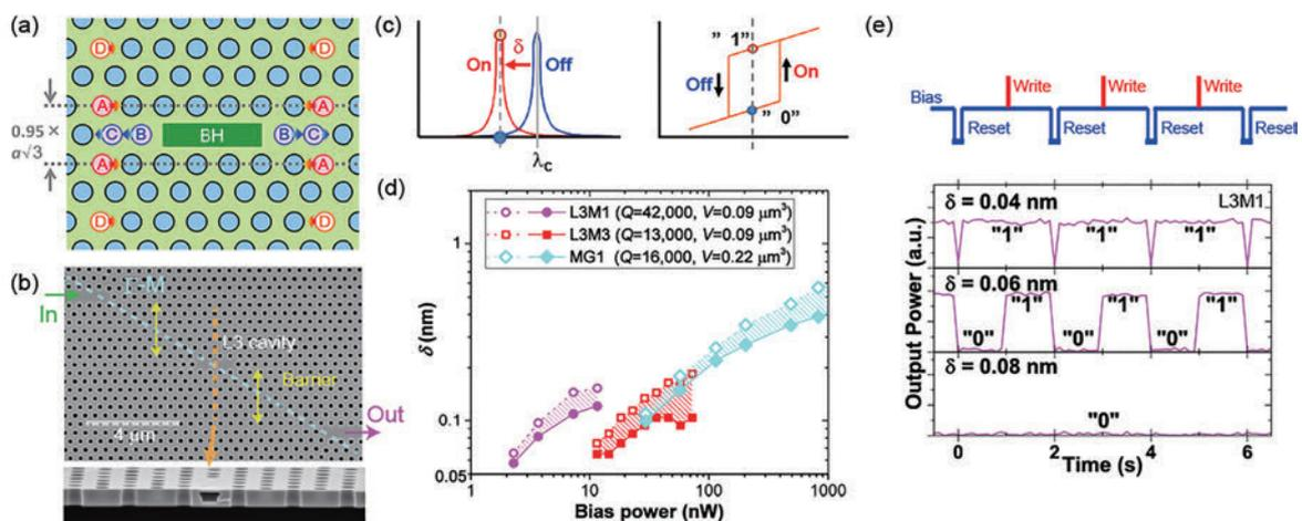
Fig. 1. (a) Design of systematically-tuned BH-L3. (Lattice constant ( $a$ ): 426 nm. Shifts:  $0.09a$ ,  $0.35a$ ,  $0.175a$ , and  $0.045a$  for A, B, C and D. BH is InGaAsP.) (b) SEM image of L3 optical memory. (c) Schematics of all-optical bistable memory operation. (d) Relation between detuning ( $\delta$ ) and bias power for memory operation. (e) Input/output waveforms in memory operation at 2.3 nW bias power.
