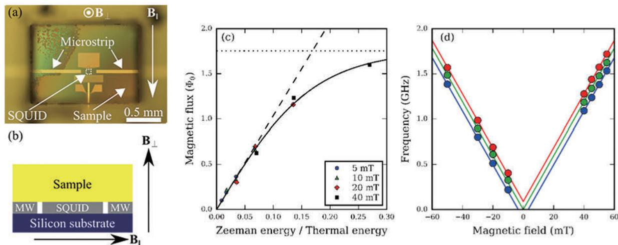
Fig. 1. (a) Optical microscope image of the sample. (b) Cross sectional view of the experimental setup. (c) Magnetization as a function of the in-plane magnetic field and the temperature. (d) Results of EPR spectroscopy.
