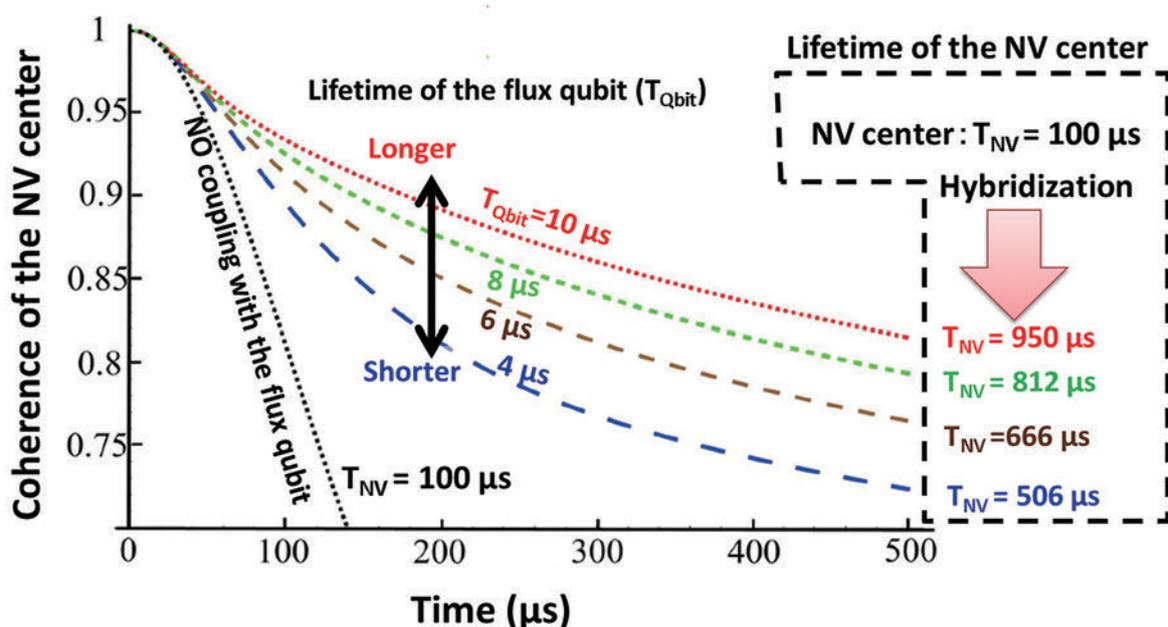
Fig. 1. Numerical simulation of the decoherence behavior of the NV center with and without coupling to the FQ. Here, the horizontal axis denotes the time and the vertical axis denotes the coherence of the NV center.
