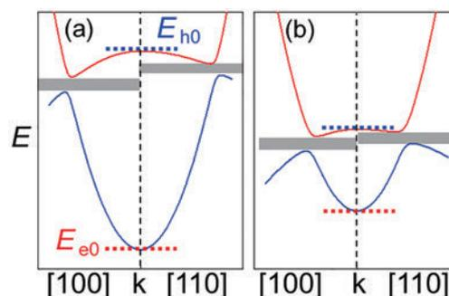
Fig. 2. Schematic illustrations of dispersion relations for (a: semimetallic) large energy band overlap case and (b: TI) small overlap case .
