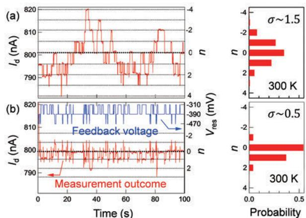
Fig. 2. Thermal-noise suppression with feedback control. (a) Thermal fluctuation of  $n$  monitored with  $I_d$  without feedback control. (b) Suppressed thermal fluctuation with feedback control.  $V_{res}$  (blue line) was modulated based on  $I_d$  (red line).
