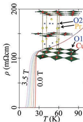
Fig. 2. Resistivity vs temperature of a coherently grown PCO thin film without annealing.
