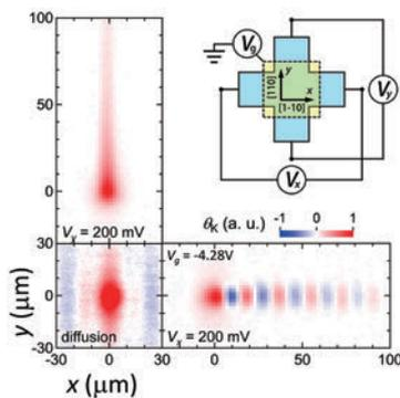
Fig. 1. Spatial distribution of diffusive and drifting spins in the PSH state. The inset shows a schematic image of the sample.
