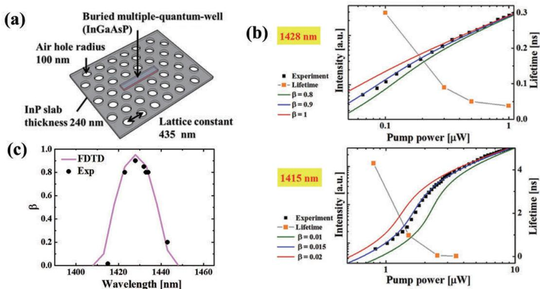
Fig. 1. (a) Schematic of L3 PhC cavity. (b) L-L curve. (c) Experimental and simulated  $\beta$ .
