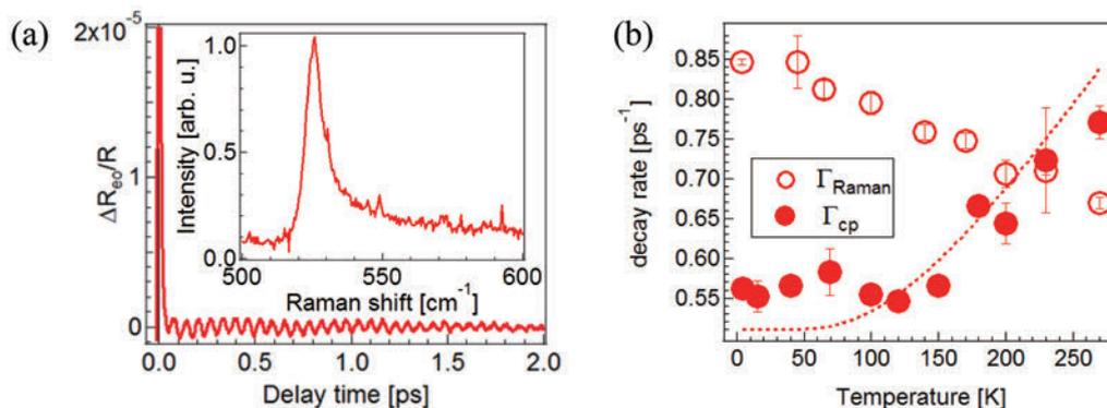
Fig. 1. (a) Time-resolved reflectivity of *p*-type Si. The inset shows the Raman spectra of *p*-type Si. (b) Temperature dependence of the phonon decay rate. The solid and open symbols correspond to  $\Gamma_{\text{cp}}$  and  $\Gamma_{\text{Raman}}$ , respectively. Dotted lines are the fits with the anharmonic decay models.
