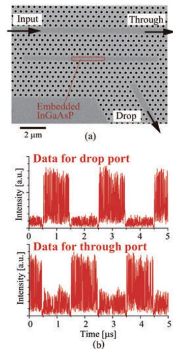
Fig. 2. (a) 1 $\times$ 2-port configuration of nanocavity. (b) Output waveforms showing the output-port-selective switching of optical packet data.
