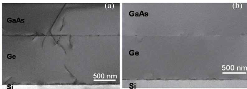
Fig. 1. Cross-sectional TEM images of (a) as-grown GaAs/Ge structure on Si substrate and (b) after TCA.
