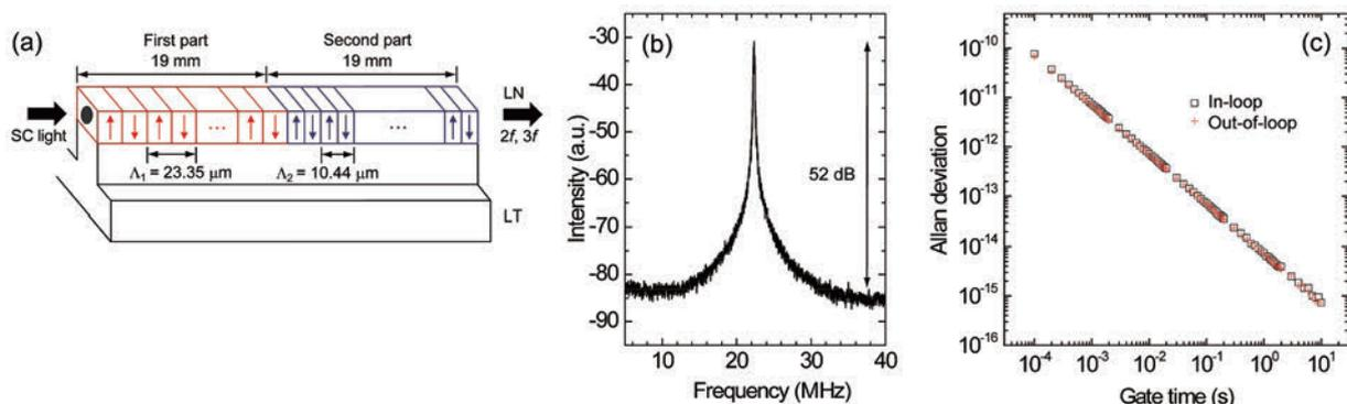
Fig. 1. (a) DP-PPLN ridge waveguide. (b) CEO beat signal. (c) Allan deviations of CEO frequencies.
