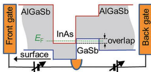
Fig. 1. Energy band profile of the InAs/GaSb heterostructure with front (surface side) and back (substrate side) gates.
