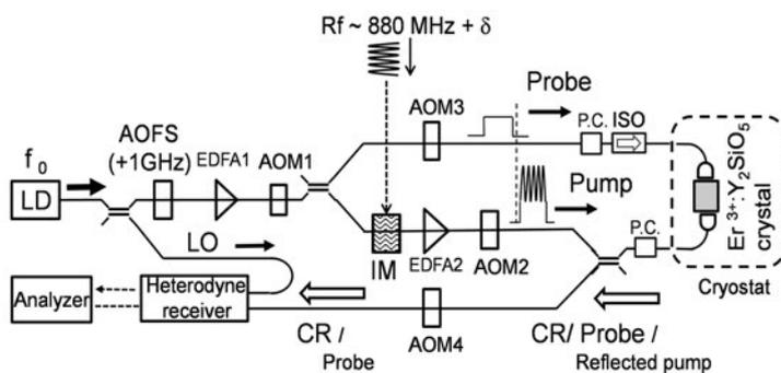
Fig. 1. Experimental configuration of the CRB spectroscopy.
