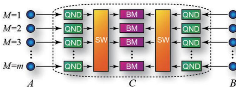
Fig. 1. All-photonic intercity QKD. The middle point  $C$  performs quantum nondemolition measurement (QND) on optical pulses sent by communicators  $AB$ . Optical switches (SW) then make only surviving photons paired, which are subjected to the Bell measurement (BM).
