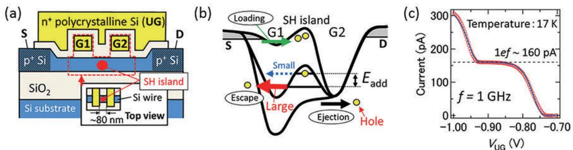
Fig. 1. (a) Schematic of the device. (b) Hole potential diagram and SH transfer mechanism. (c) Measurement data for the high-speed SH transfer and a fit.
