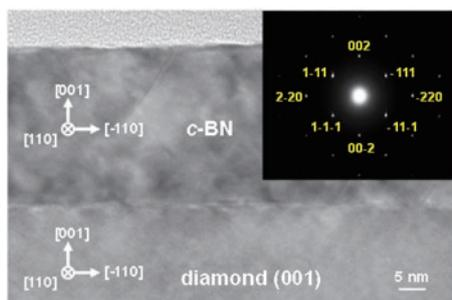
Fig. 2. Cross-sectional TEM image and SAED pattern of epitaxial *c*-BN(001) film.
