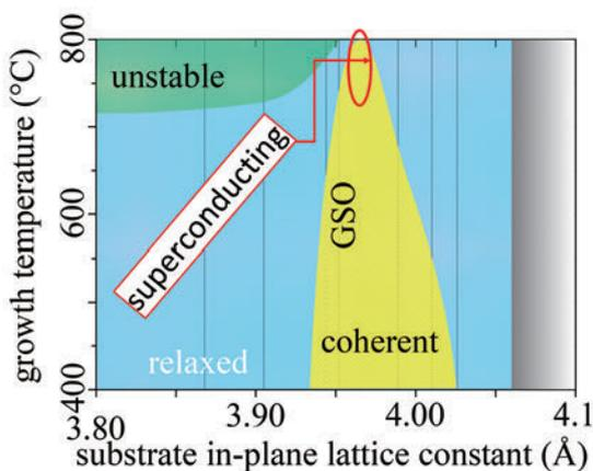
Fig. 1. Synthesis conditions for coherently grown PCO thin films.
