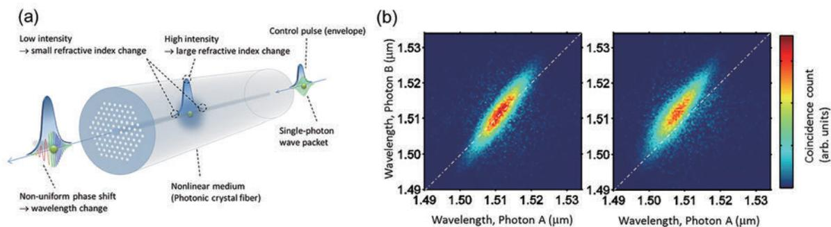
Fig. 1. (a) The illustration of the scheme. (b) Reshaping the non-classical frequency correlation between photons. In the experiment, first, photon pairs were created via an optical process called parametric down conversion (left). Then the wavelength of “photon A” was blue shifted with our scheme. As a result, the overall spectral correlation was also blue shifted (right).
