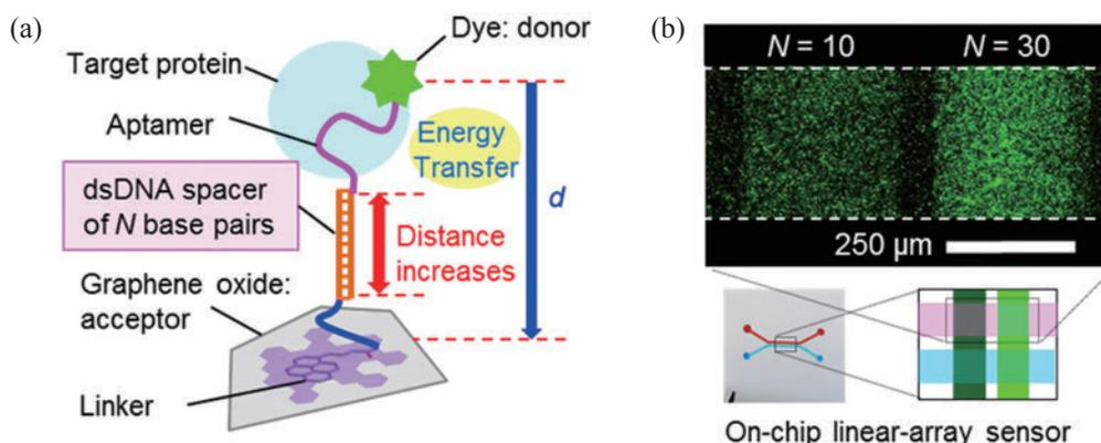
Fig. 1. (a) Molecular design of the probe (ii) for enhancing sensitivity of the aptasensor. (b) Quantitative comparison of enhancement effect depending of the spacer length.
