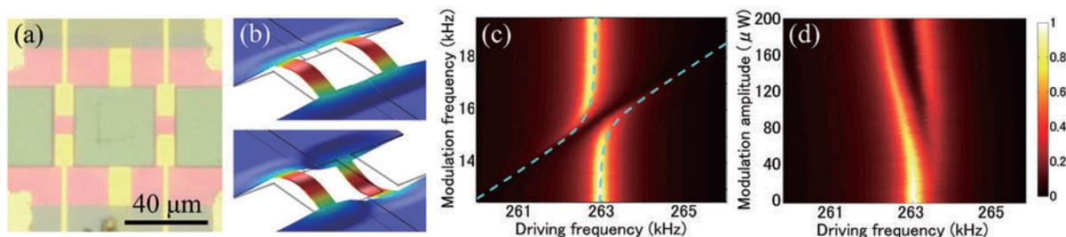
Fig. 1. (a) Microscope image of two mechanical resonators. (b) Schematic image of the symmetric and anti-symmetric modes calculated by the finite element method. (c) Modulation-frequency dependence and (d) modulation-amplitude dependence of anti-symmetric mode. Blue dotted lines show calculated peak frequencies.
