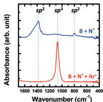
Fig. 1. FT-IR spectra of BN films grown with and without  $Ar^+$  irradiation.
