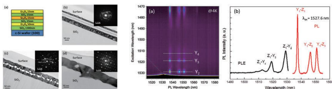
Fig. 1. (Left) Fabricated structures, (Middle) PLE color plot measured at 4 K obtained from the sample annealed at 1250°C. (Right) PLE and PL spectra at 4K.
