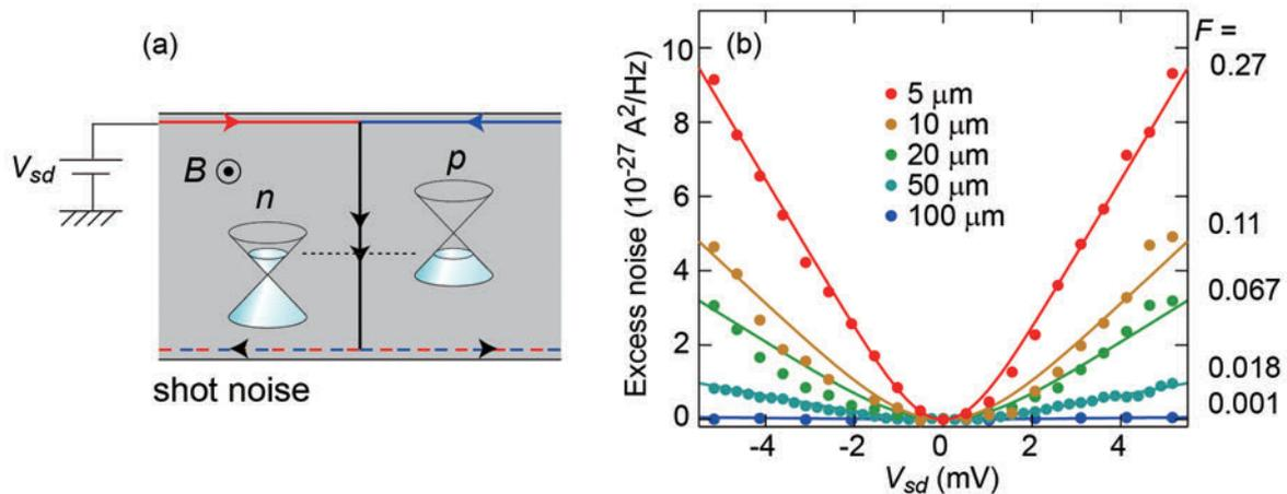
Fig. 1. (a) Counter-circulating electron and hole edge modes in a bipolar graphene quantum Hall effect regime. (b) Shot noise as a function of the source-drain bias for the samples with different  $p$ - $n$  junction length.
