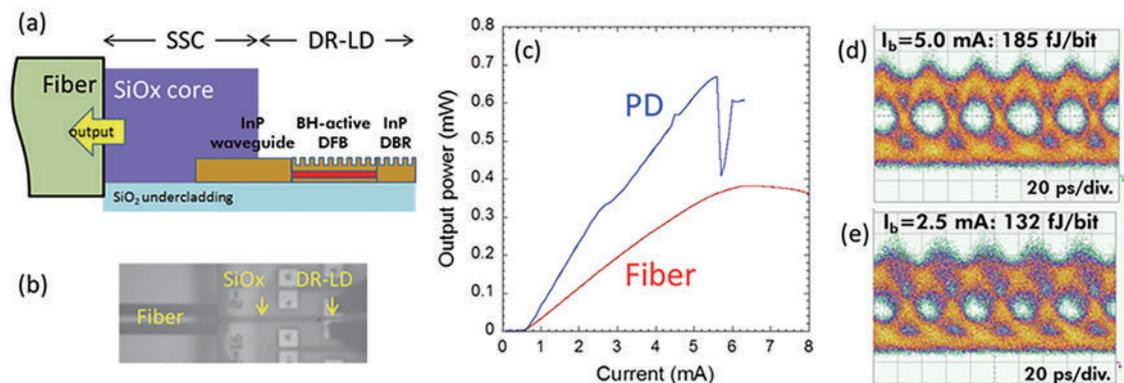
Fig. 1. (a) Schematic device structure. (b) Top-view image of a fabricated device. (c)  $I$ - $L$  characteristics. (d) (e) Eye diagrams for 25.8-Gbps NRZ direct modulation with  $I_b$  of 5.0 mA and 2.5 mA.
