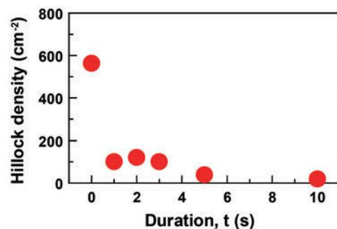
Fig. 2. Hillock density on N-face GaN (000 $\bar{1}$ ) film surfaces plotted as a function of  $t$ .
