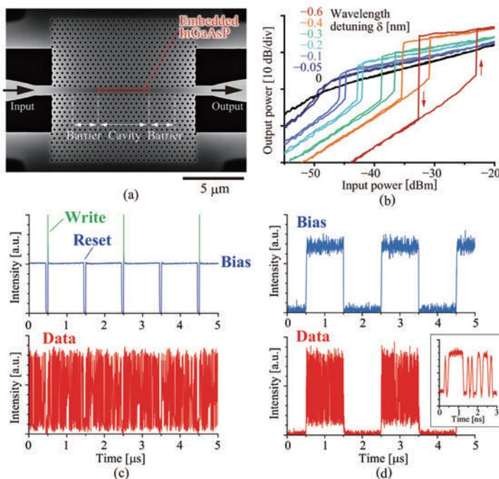
Fig. 1. (a) Photograph of photonic crystal nanocavity. (b) Hysteresis curves on optical input/output characteristic. (c) Input optical waveforms. (d) Output waveforms showing the gate switching of optical packet data.
