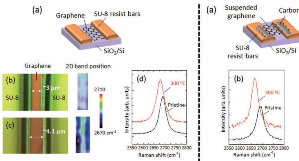
(Left) Fig. 1. (a) A schematic of GG sample. Optical microscopy images and the corresponding Raman 2D peak position maps (b) before and (c) after annealing at 300°C. (d) Raman spectra before and after annealing. (Right) Fig. 2. (a) A schematic of SG sample. (b) Raman spectra before and after annealing.
