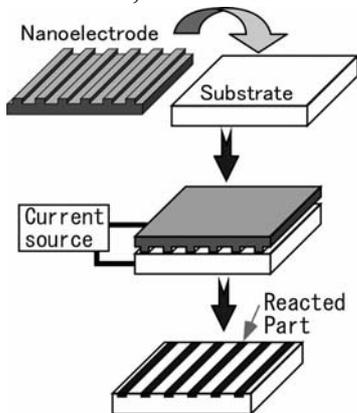
Fig. 1 Nanoelectrode lithography
