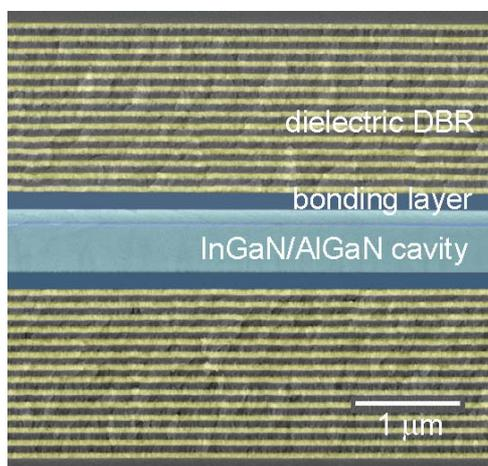
Cross-sectional SEM image of microcavity
