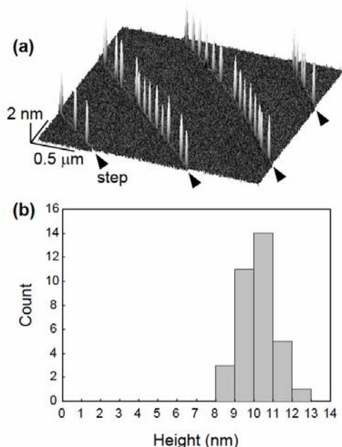
Fig. 1. AFM image of 3D islands and their height distribution.
