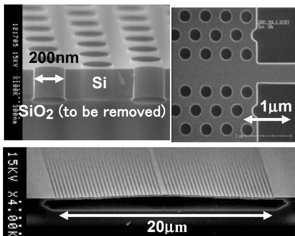
Fig. 1. SEM images of Si PCSs fabricated in this study.
