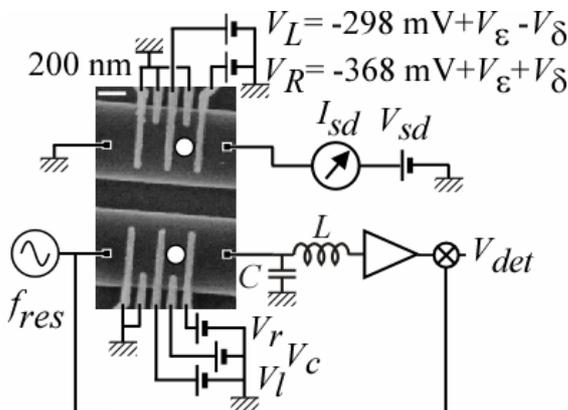
Fig. 1. Measurement system and an electron counting device.
