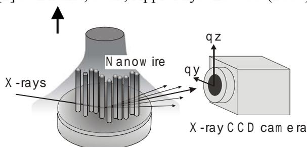
Fig.1 Experimental layout of GISAXS.
