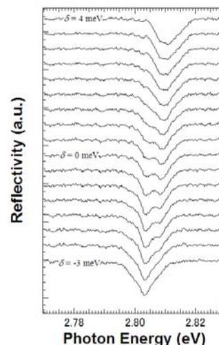
Fig. 3. Formation of cavity polariton.
