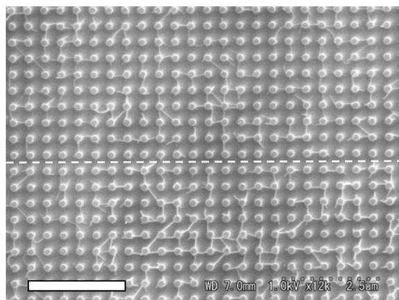
Fig. 2. SEM image of the suspended SWNT network after the selective removal procedure. The electron beam was scanned along the dashed line. Scale bar: 2.5  $\mu\text{m}$ .
