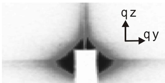
Fig.2 GISAXS image after nanowires formation ( $T_s=400$  )
