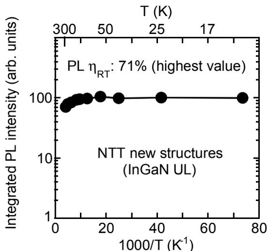
Fig. 1. Arrhenius plots of integrated PL intensity for InGaN QWs on an InGaN UL
