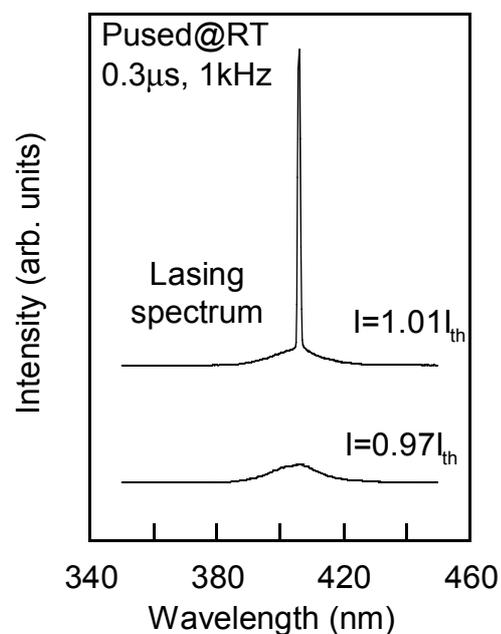
Fig. 2. Emission spectra obtained from an InGaN-based HCSEL below and above the lasing threshold.
