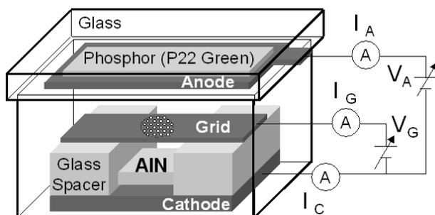
Fig. 1. Schematic diagram of display structure using heavily Si-doped AlN.
