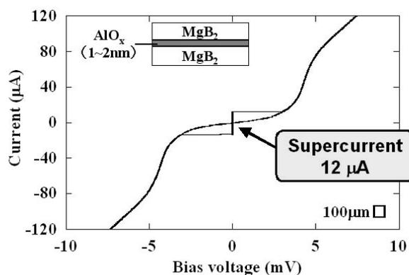
Fig. 1: Typical current-voltage characteristics of the MgB<sub>2</sub> tunnel junction measured at 4.2 K.
