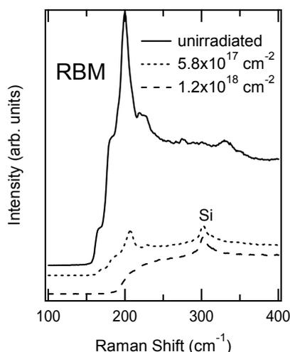
Fig. 1. Raman spectra of SWNTs before and after electron irradiation.
