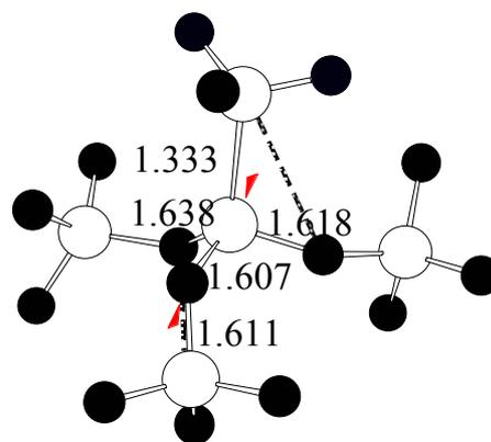
Fig. 2. Structure of high-density oxide regions with oxygen vacancies
