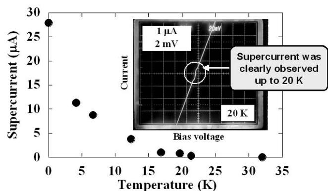
Fig. 2: Temperature dependence of supercurrent of the MgB<sub>2</sub> tunnel junction. The inset shows current-voltage characteristics measured at 20K.
