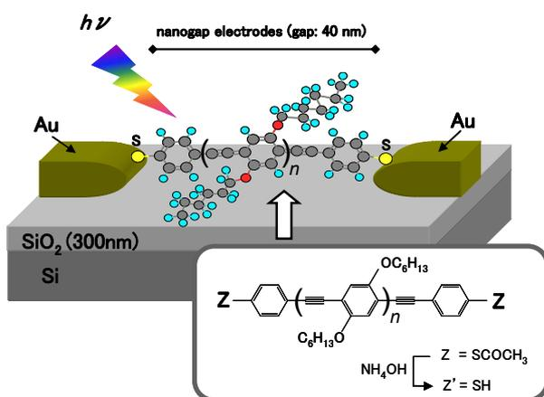
Fig. 1. Molecular structure of TA-PPE and nanodevice structure
