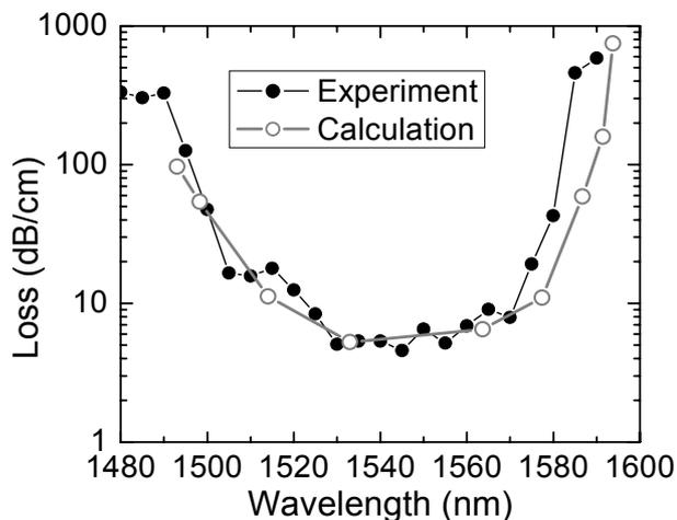
Fig. 2. Measured and calculated loss spectra of PCS waveguides.
