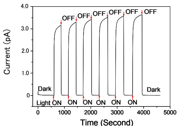
Fig. 2. Photoresponse characteristics of the nanojunction device (white light, 52 mW)
