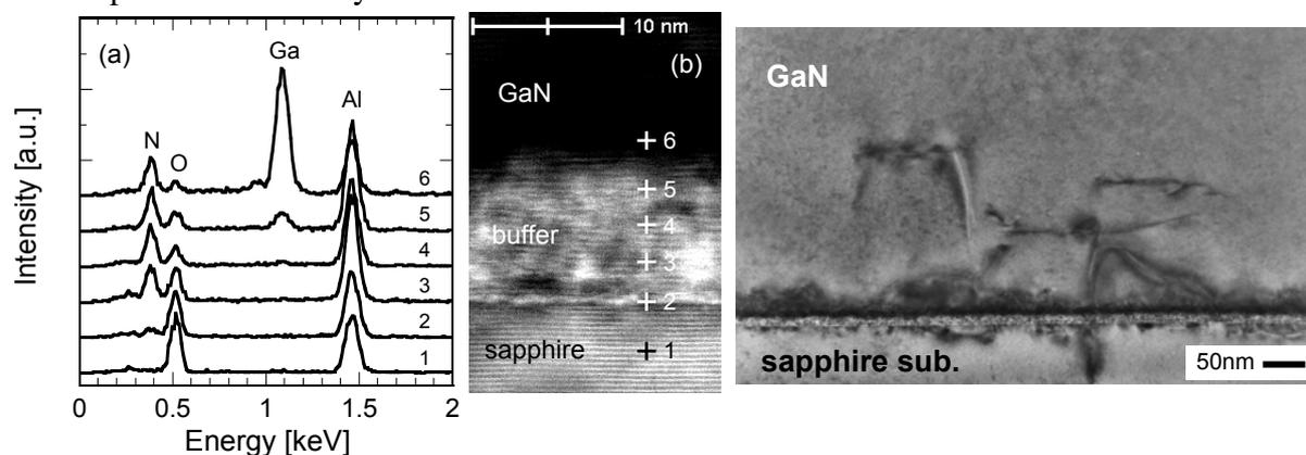
Figs. 1. (a) The EDS profiles and (b) the cross-sectional TEM image at the interface between the sapphire substrate and the GaN layer, respectively.
