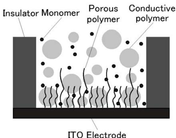
Fig. 1 Structure of a polymer electrode
