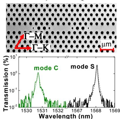
Fig. 1. Electron microscope image of the silicon PhC nanocavity (top). Linear transmission spectrum (bottom).
