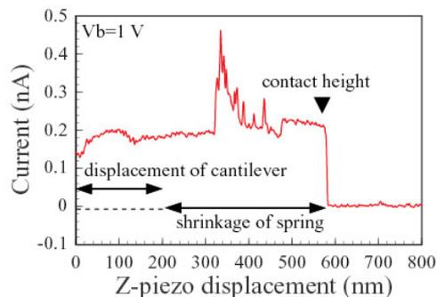
Fig. 2. Displacement dependence of probe current. Voltage of the sample (Au film) is 1V.
