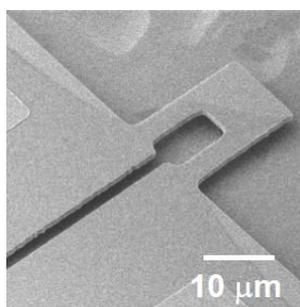
Fig. 1 SEM image of a fabricated piezoresistive cantilever.
