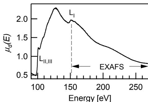
Fig. 1. Example of Si-absorption spectrum.
