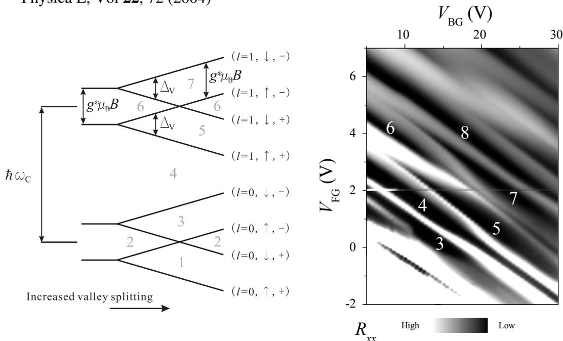
*Left:* A schematic diagram of Landau levels with increased valley-splitting.
