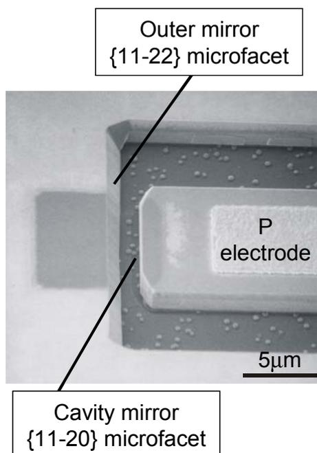
Fig. 1. Bird's-eye-view SEM photograph of an InGaN-based HCSEL.
