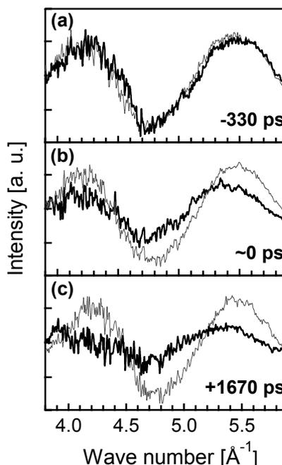
Fig. 2. Transient EXAFS spectra with (thin black line) and without (thick gray line) laser irradiation.
