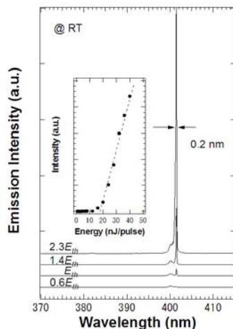
Fig. 2. Lasing by optical pumping.
