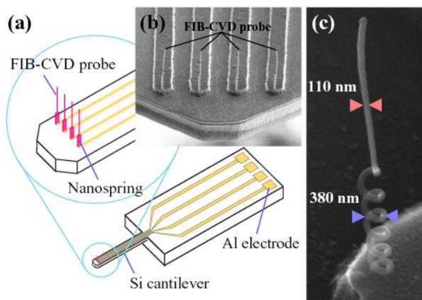
Fig. 1. (a) Schematic of four-point probe on Si cantilever. (b) SEM micrograph of integrated FIB-CVD multi-probe. (c) Magnified image of carbon probe with nano-spring on Al electrode.
