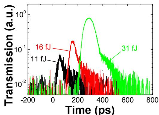
Fig. 2. Recorded switching operation of the signal waveform as a function of the control pulse energy.
