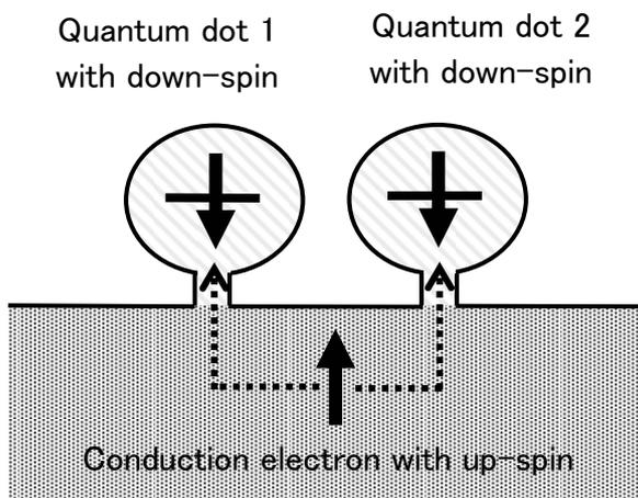
Figure: Two quantum dots coupled to the conduction electron system. Electron spins in two dots are aligned in the downward direction when the conduction electron with opposite (up) spin jumps back and forth between two dots.
