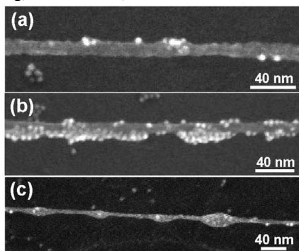
Fig. 2. SEM images of CNT/Au hybrids [(a),(b)] and CNT/DNA/Au hybrid (c).
