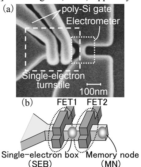
Fig. 1. (a) SEM image. (b) Schematic view of the single-electron turnstile.
