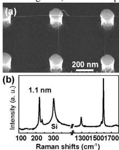
Fig. 1. Suspended SWNTs from Co-ferritin.
