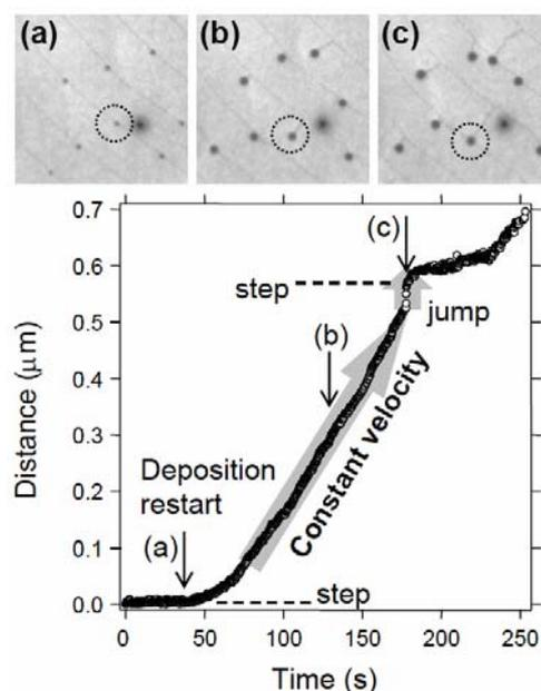
Fig. 2. The moving distance of the island indicated by the dotted circle in LEEM images (a)-(c) as a function of time.
