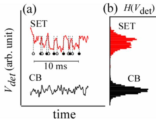
Fig. 2. Single-electron counting (SET) and background noise (CB)
