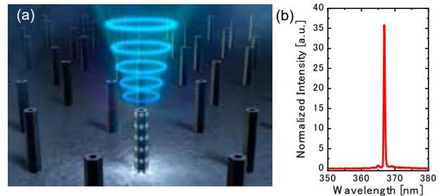
(a) Schematic diagram of hollow nanowire lasers.
