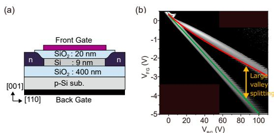
(a) Schematic diagram of the device.
