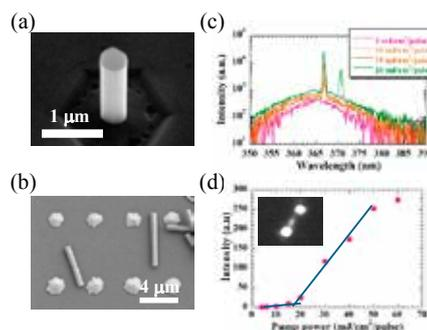
(a) Bird's eye-view scanning electron microscope image of nanowires after etching. (b) Nanowires dispersed on a sapphire substrate. (c) Photoluminescence spectra from a single nanowire at various pump powers. (d) Emission intensity as a function of excitation intensity. Strong emission from the end facets of the nanowire can be seen in the inset image.
