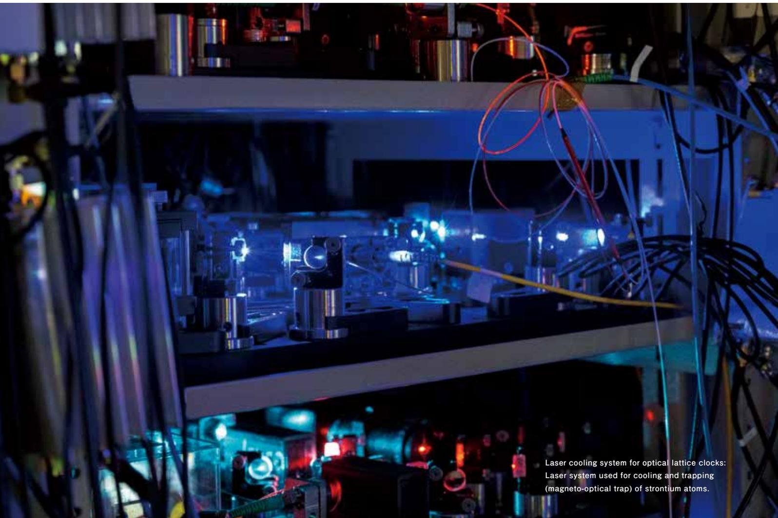
Laser cooling system for optical lattice clocks:
