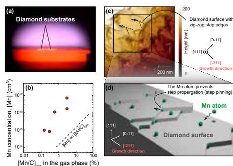
(a) Photograph taken during diamond growth by microwave plasma CVD. (b) Mn concentration in diamond as a function of [Mn/C] ratio in the gas phase. (c) AFM image of Mn-doped diamond (111) surface. (d) Schematic growth mechanism of Mn-doped diamond (111) layer.
