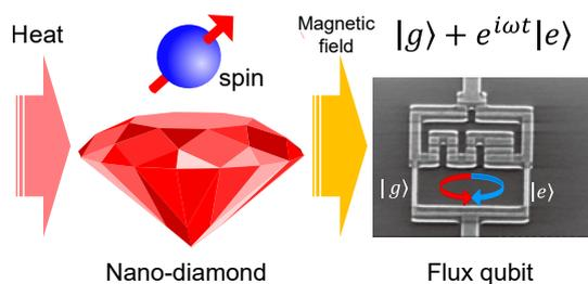
The polarization of the electron spin in the nanodiamond changes due to heat from the object to be measured. The magnetic field change caused by the polarization change is detected using the phase of the superconducting flux qubit.
