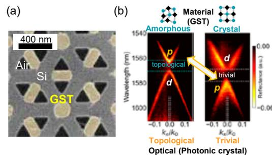
(a) SEM image of the fabricated topological photonic crystal. Nanometer-sized GST blocks are precisely deposited on the silicon photonic crystal.
