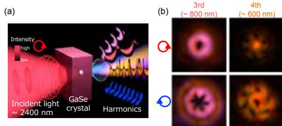
(a) Schematic diagram of high-harmonic generation in a crystalline solid.
