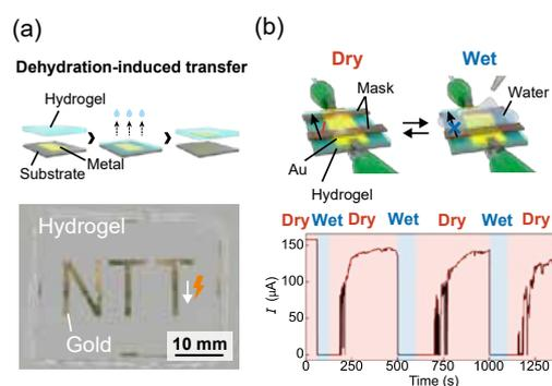
(a) Adhesion to metal films can be achieved with arbitrary shapes. (b) The metal transferred onto a fully dehydrated hydrogel becomes electrical wiring that changes conductivity as the gel swells and shrinks in response to ambient moisture.
