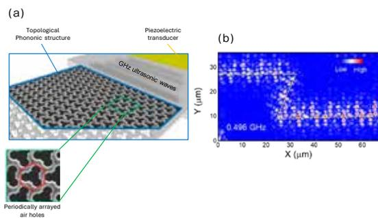
(a) Schematic diagram and SEM image of a GHz topological phononic structure.
