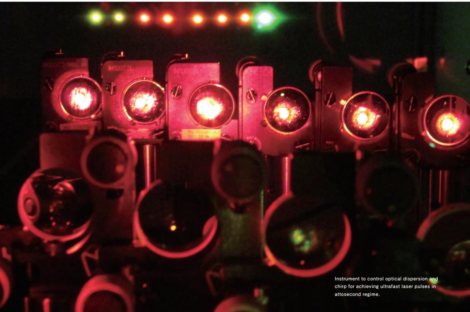
Instrument to control optical dispersion and chirp for achieving ultrafast laser pulses in attosecond regime.
