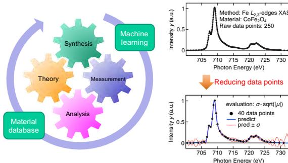
(Left) Research cycle for the development of novel materials. (Upper right) Spectrum, which consists of 250 data points, obtained by the conventional spectroscopy. (Lower right) Spectrum predicted by GPR with 40 data points.
