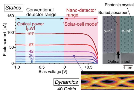
Photonic-crystal nano-detector operating fast in solar-cell mode
