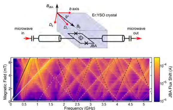
(Top) Schematic diagram. (Bottom) Observed ESR spectra.
