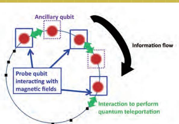
Schematic illustration of a quantum teleportation based magnetic field sensor.
