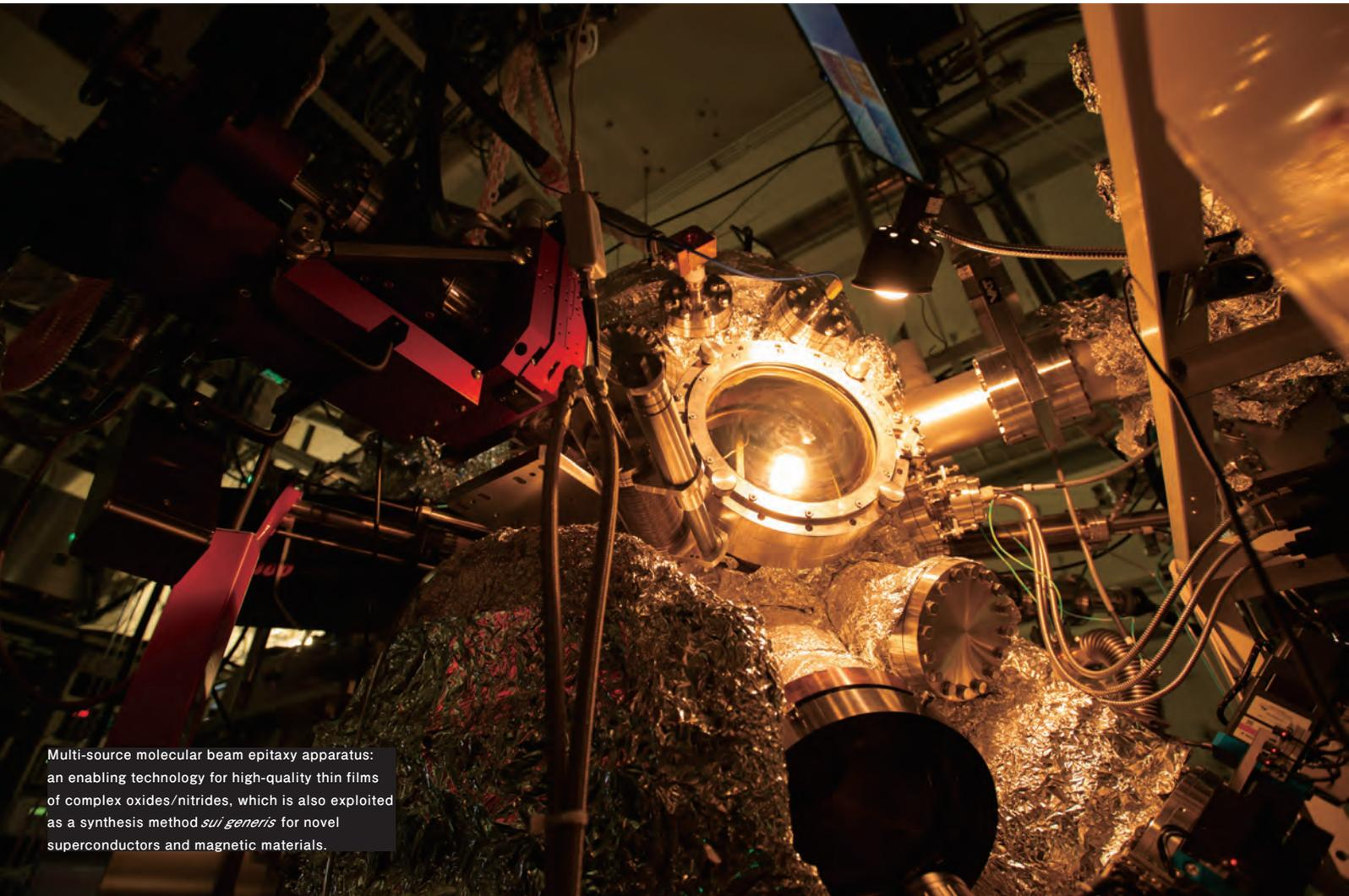
Multi-source molecular beam epitaxy apparatus: an enabling technology for high-quality thin films of complex oxides/nitrides, which is also exploited as a synthesis method *sui generis* for novel superconductors and magnetic materials.
