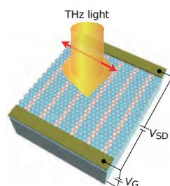
Experimental setup. Graphene is transferred on a SiO<sub>2</sub>/Si substrate (light blue) covered with a micro-ribbon array of a self-assembled graphene/SiO<sub>2</sub> micro-ribbon arrays (SAM: orange).
