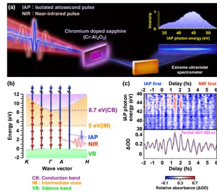
(a) Transient absorption attosecond spectroscopy, (b) Energy band structure of Chromium doped Sapphire, (c) Attosecond electron interferogram
