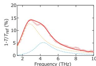
Extinction spectrum. Observed two peaks correspond to excitations of plasmons localized in the graphene/SAM and graphene/SiO<sub>2</sub> micro-ribbon arrays.
