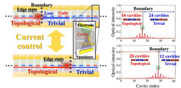
Controllable photonic topological insulator and boundary edge states
