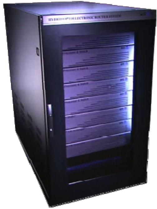
Hybrid optoelectronic packet-switched router prototype
