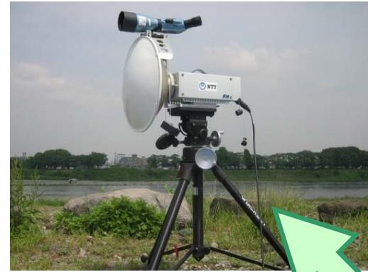
Real-time millimeter-wave imaging system
